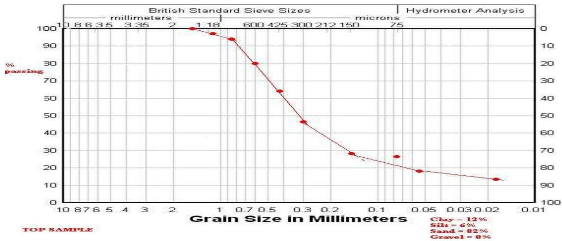
Figure 4: Sieve Analysis from Top Sample
